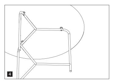
Gradually tighten all three screws to ensure a secure and even fit.
