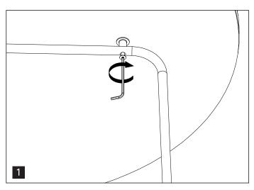
Place the tabletop onto the base. Align one of the three screw holes with a spacer. Insert and secure the screw, but do not fully tighten it yet.
