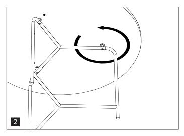
Gently rotate the tabletop until the remaining two screw holes align with their corresponding spacers.
