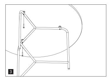
Insert and secure the remaining two screws, but do not fully tighten them yet
