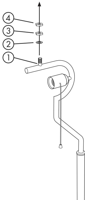
Install the ring on the shade. Place the shade on top of the tube spacer. Install the washer (2) and nut (3) and tighten the nut. Install and tighten nut (4).
