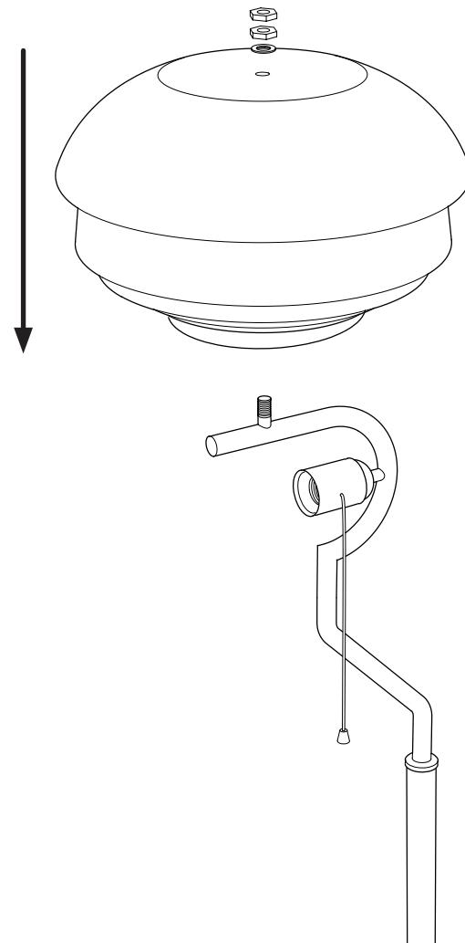
Install the top of the shade by turning it clockwise.
