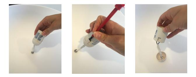
4. Remove the rest of the damaged shade and replace it with the new one. Mount the socket on to the cord again and screw it back on to the marble base.
